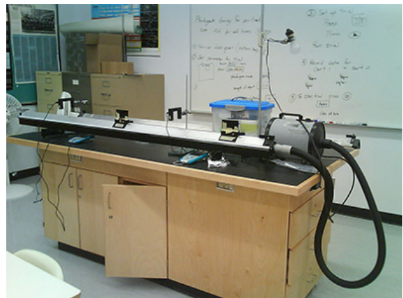
"Air Track with photo-gates and a reverse vacuum" by Bhavesh Chauhan is licensed under CC BY 3.0
