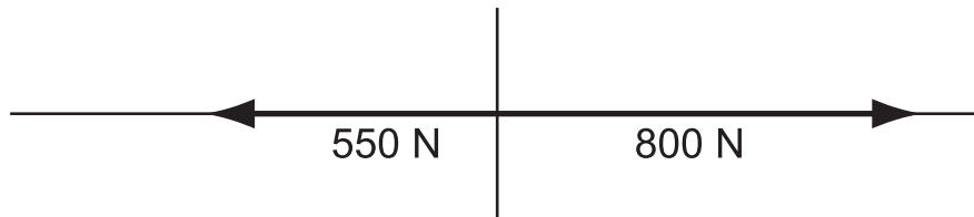
Figure 1.3: Two forces acting in opposite directions
