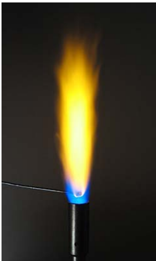
Sodium heated in a flame (photo by Swm, licensed under CC BY-SA 3.0)
